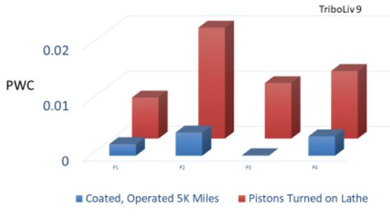
**Figure 8:** Piston to Wall Clearance (PWC) was corrected by AAPC after turning piston skirts to undersize straight on a lathe, coating them to fit. Coated pistons operated 5000 miles before remeasuring.
