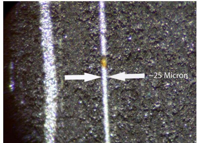
**Figure 5B:** Slick+ AAPC coated piston skirt with trapped crystallite particle
