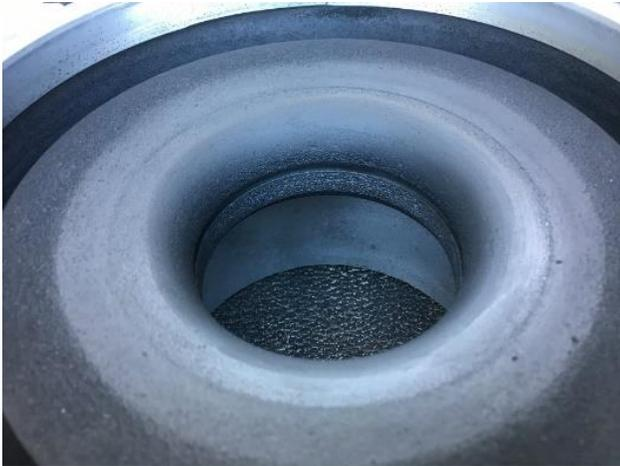
**Figure 11:** Coated compressor housing after 150,000 miles in service
